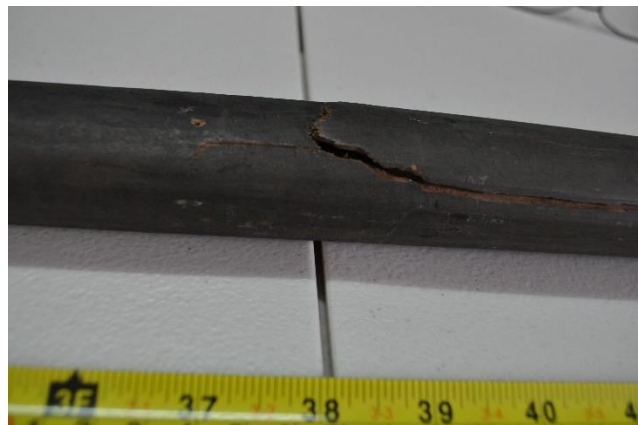
2090a – oar loom showing significant splitting
