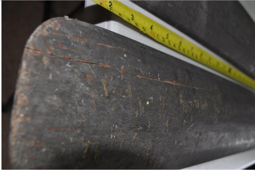
Oar 2090a showing splitting along the blade
